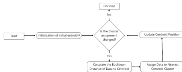
Figure 1: K-Means Implementation Process Flowchart
