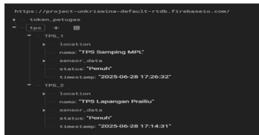
Fig. 7: Firebase Realtime Database Data Structure
