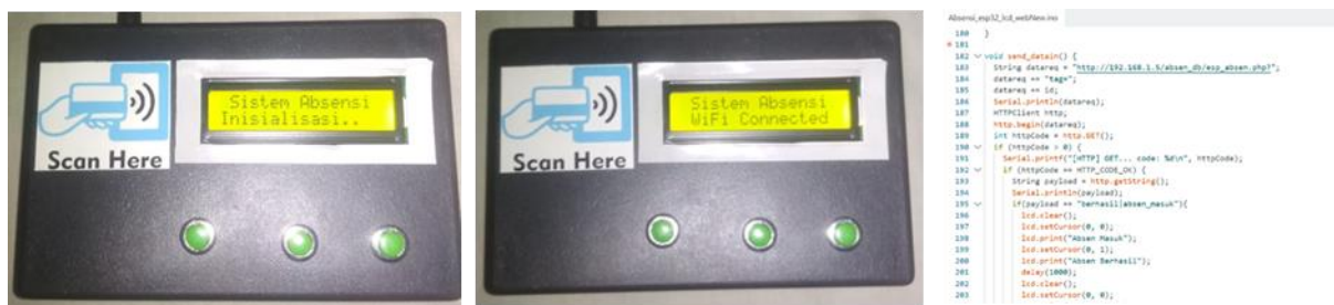
Fig. 8: Connectivity Testing of Installed Devices
