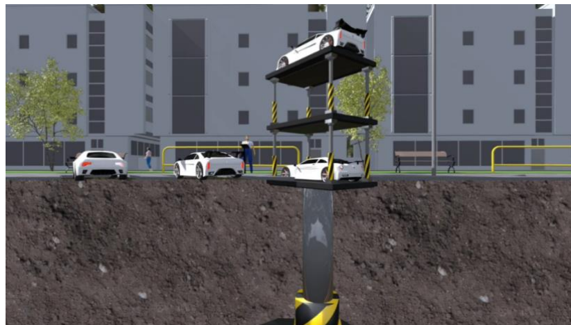
Fig. 5: Underground parking lift system perspective view
