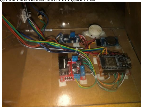
Figure 6: ESP32 Hardware Design and Other Components
