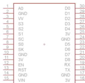
Figure 3: The NodeMCU ESP8266 circuit
