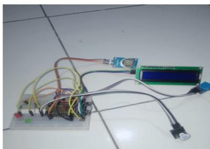
Fig. 4: Overall hardware implementation of the IoT-based air quality monitoring system
