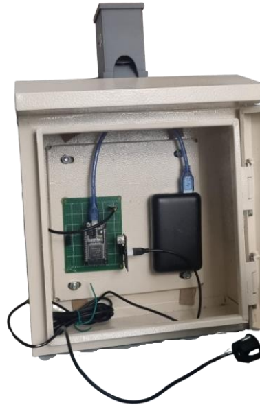
Figure 3: Hardware implementation of the monitoring system within the protective enclosure
