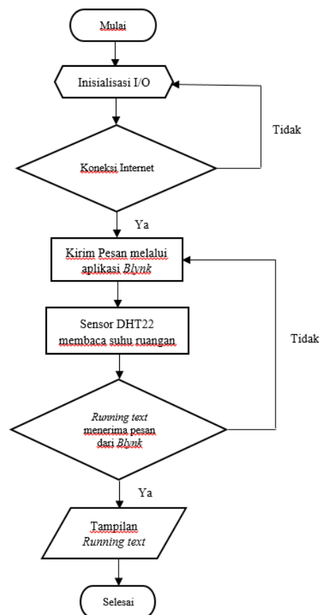
Fig. 3: Flowchart System Control
