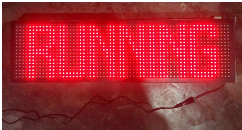
Fig. 11: Display of Running Text After Sending Text via Blynk
