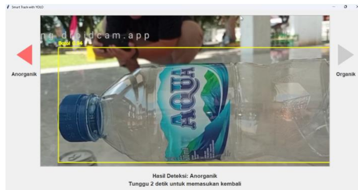
Fig. 10 Bottle detection testing
