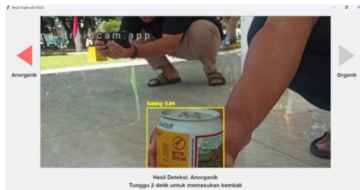
Fig. 11 Drink can detection testing
