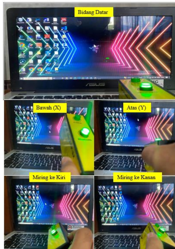
Figure 11: Results of the ESP32 and MPU6050 Based Air Mouse Tool
