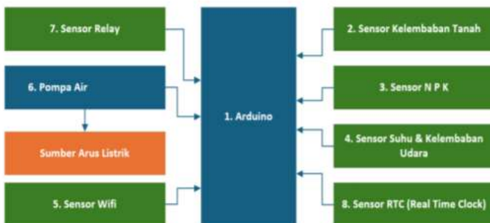
Gambar 3. Diagram Alir Sistem Monitoring Lahan Pertanian Berbasis IoT
